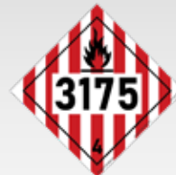
Solids containing flammable liquid, n.o.s. 4" - DC-ISO-251600 10.75" - DC-ISO-251601
